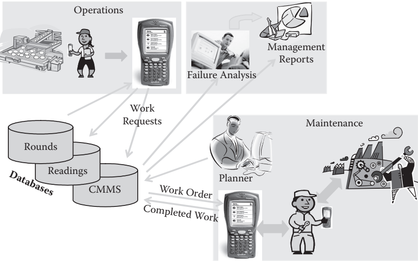
FIGURE 5.7 Field operations/maintenance of tomorrow.
